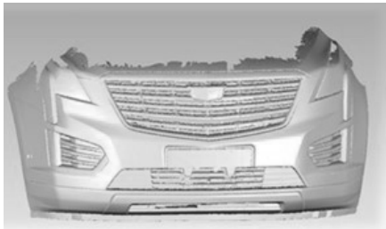
Scan the point cloud data
